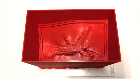
Fig. 13. 3D printed walls used for the silicone pouring procedure.
